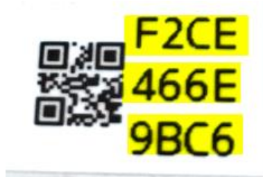
Figure 39. Sticker on device that shows QR code and corresponding MAC address
