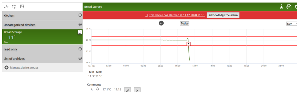
Figure 11. A temperature alarm displayed in the service.
